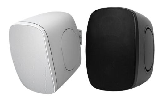
CX-DSP6060 is an outdoor waterproof wall mounted speaker, which features IP65 waterproof level and inverted-phase design. It consists of tweeter and woofer units for clear and bright sound. The speaker box is made of ABS engineering plastic and the mesh is made of aluminum material for stable and reliable operation in indoor and outdoor environments.
